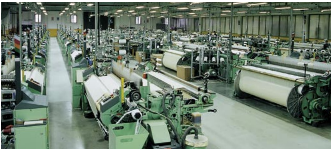
DORNIER Rapier and Air-jet weaving machine park in the Varallo, Italy, factory
