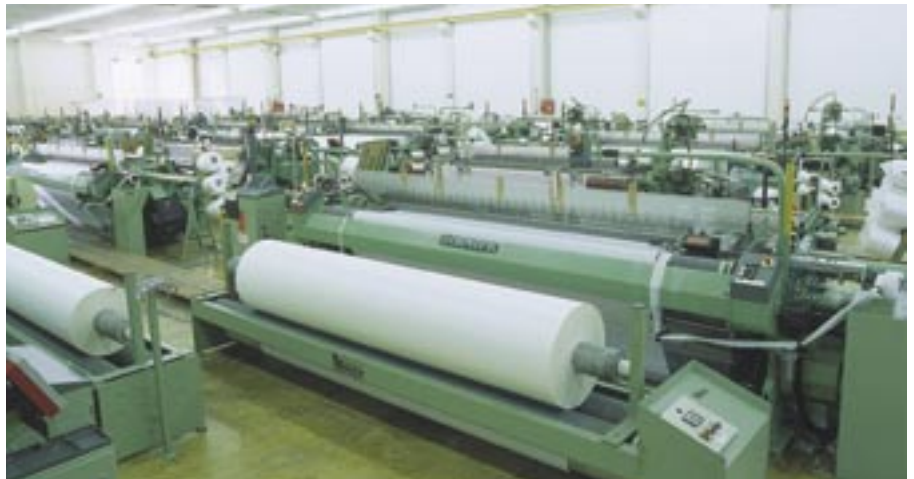
DORNIER Rapier weaving machine system for production of industrial textiles in the Rudersdorf factory, Austria
