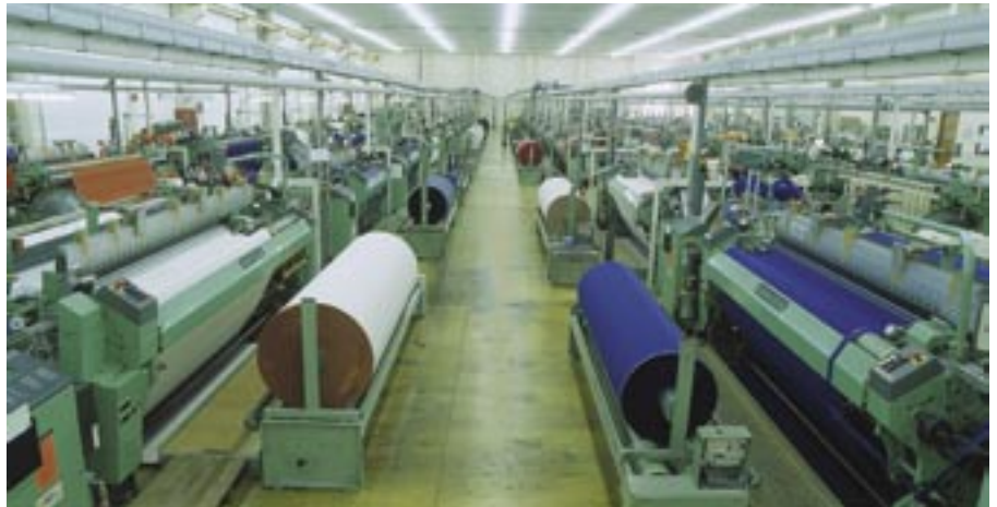
DORNIER Air-jet weaving machine system for production of sunshade textiles in the Rudersdorf factory, Austria
