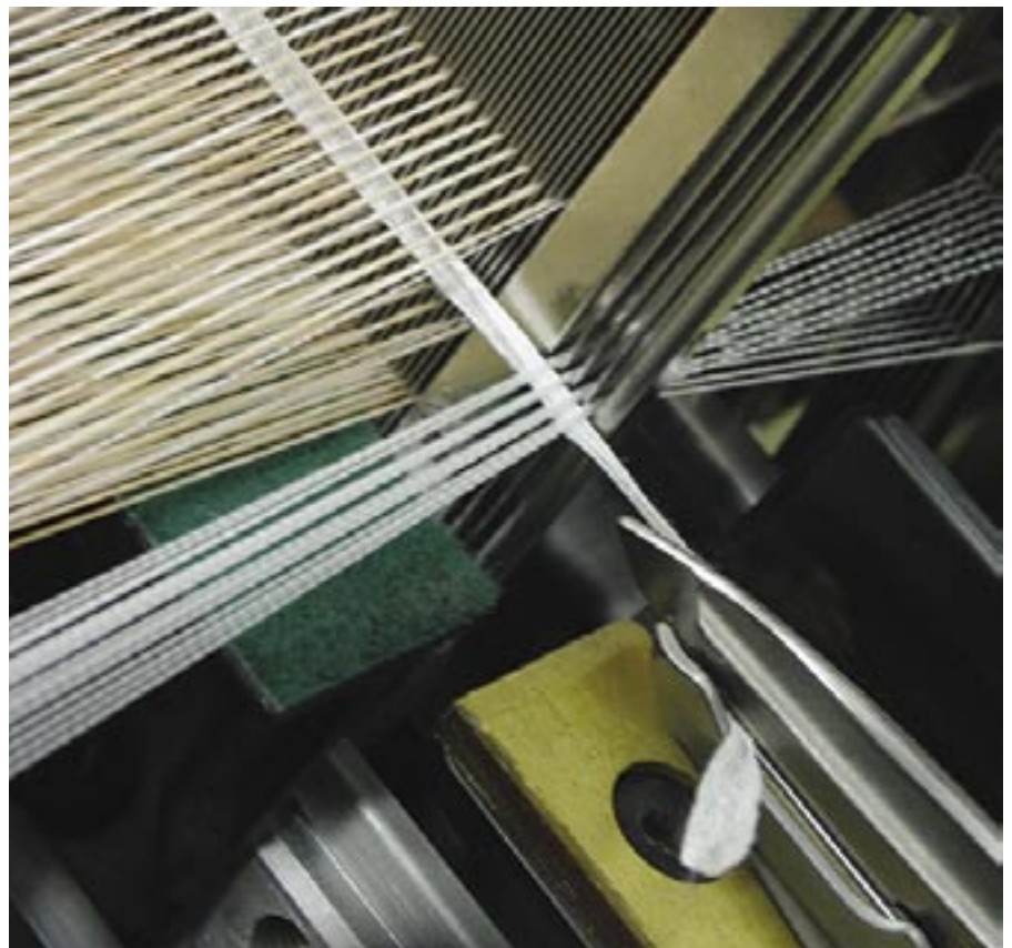
Open-shed filling insertion on DORNIER Rapier Weaving Machine
