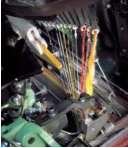
12 color filling selector on the rapier weaving machine
