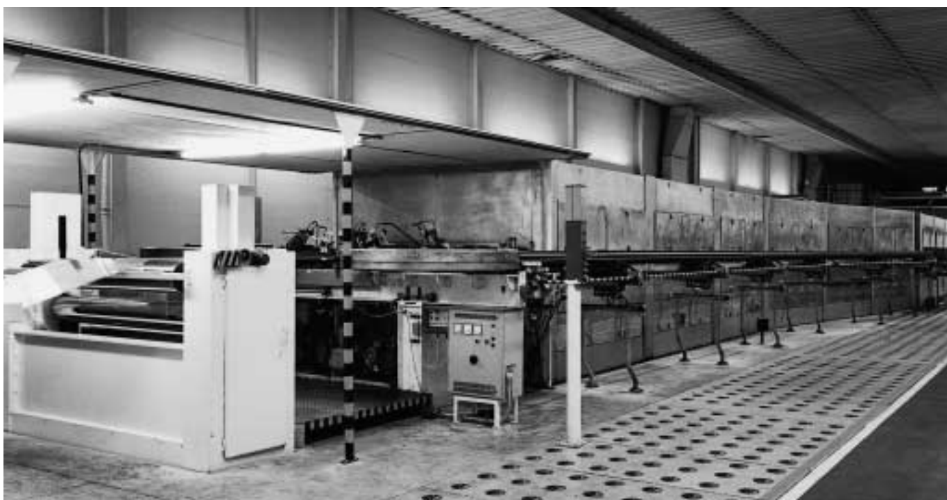
View of a DORNIER transverse stretching machine, part of a complete film stretching machine
