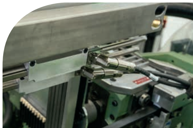
Linear motors for sideways displacement of the additional thread systems
