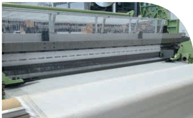
Multiaxial fabric with two additional thread systems
