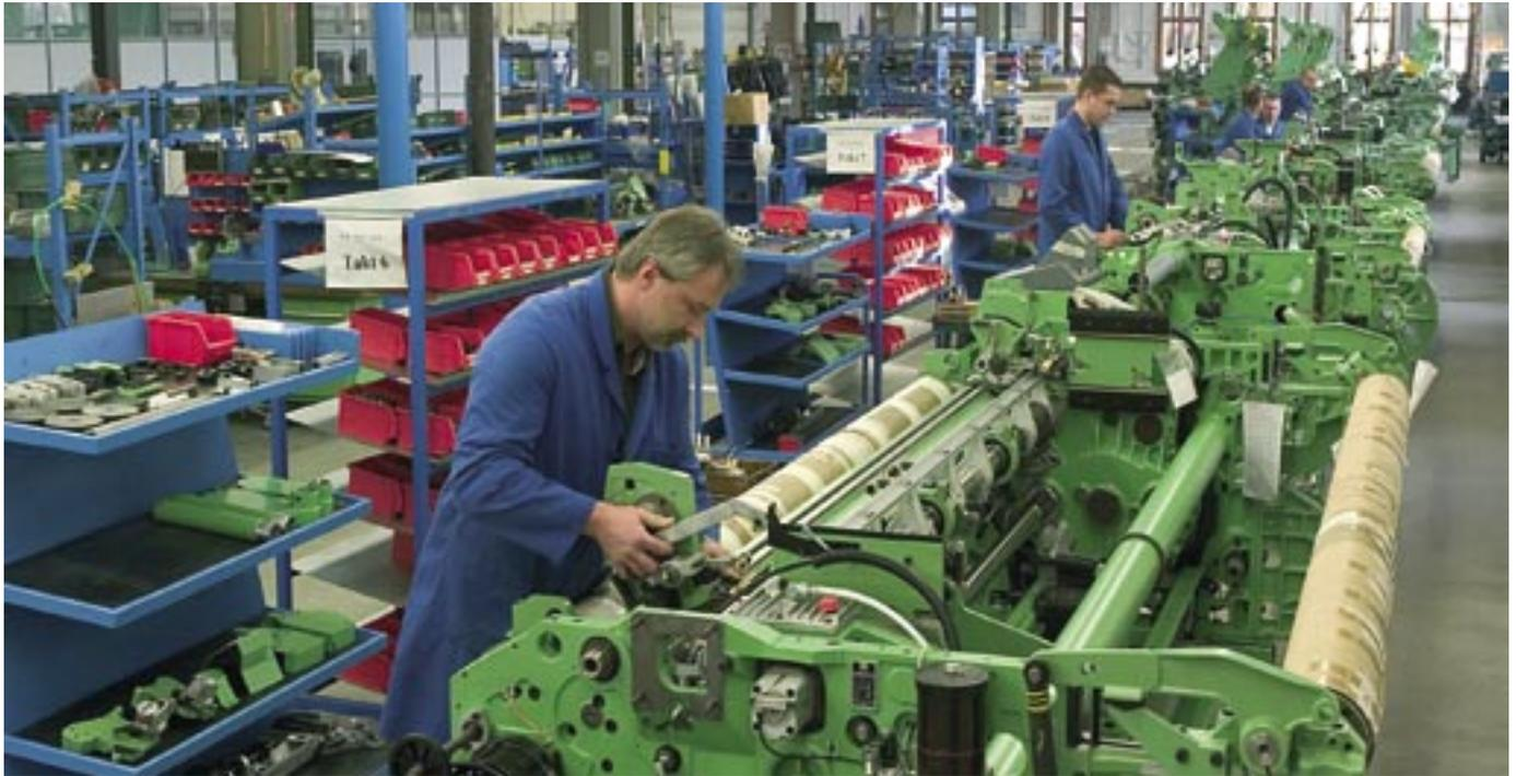
Reorganized weaving machine assembly line according to the flow principle
