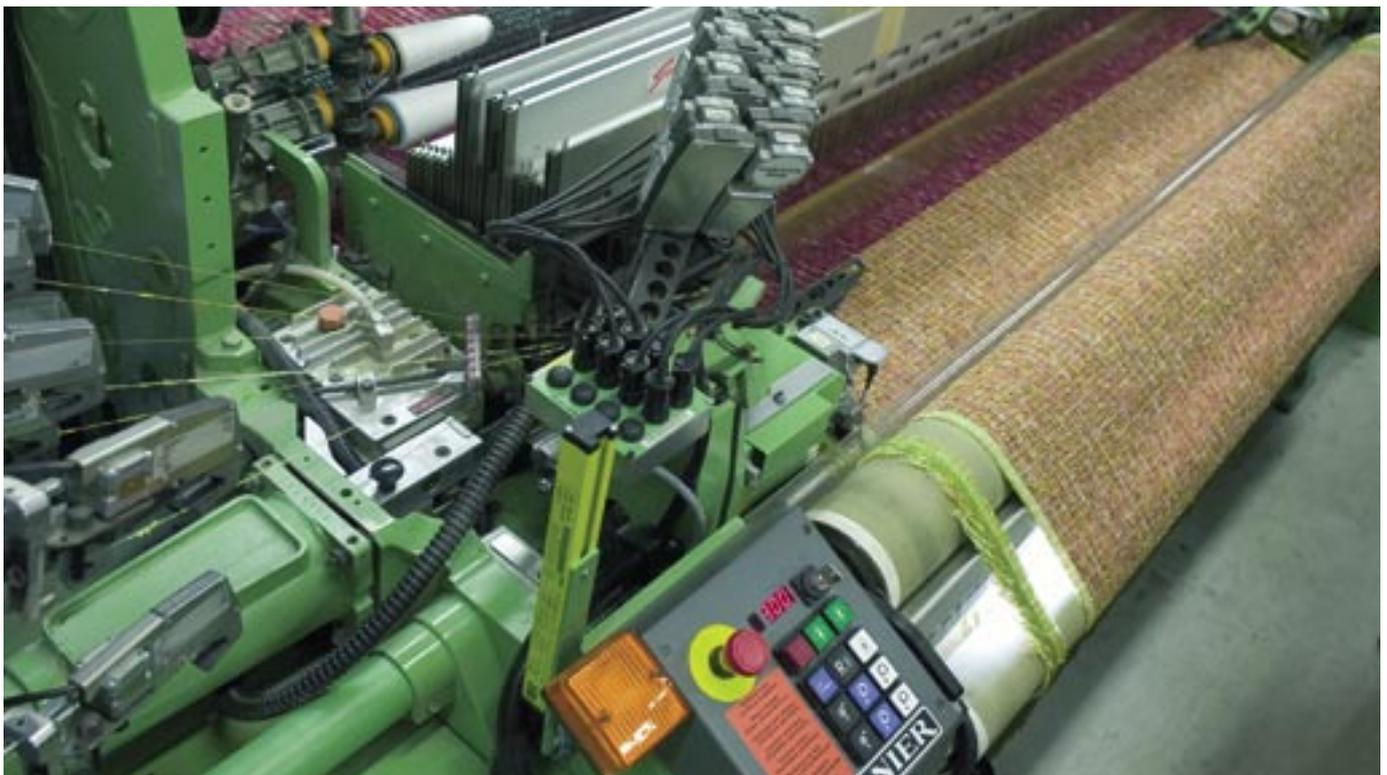
Feed side of DORNIER rapier weaving machines with patented AirGuide® as well as the newly designed control housing
