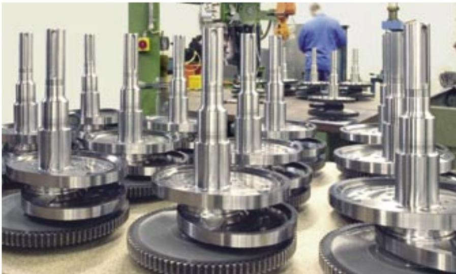
Highest manufacturing precision for conjugate cam packages for weaving machine gearboxes
