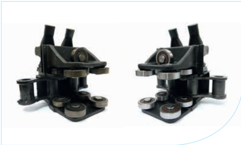
Clip before and after overhauling in a DORNIER workshop
