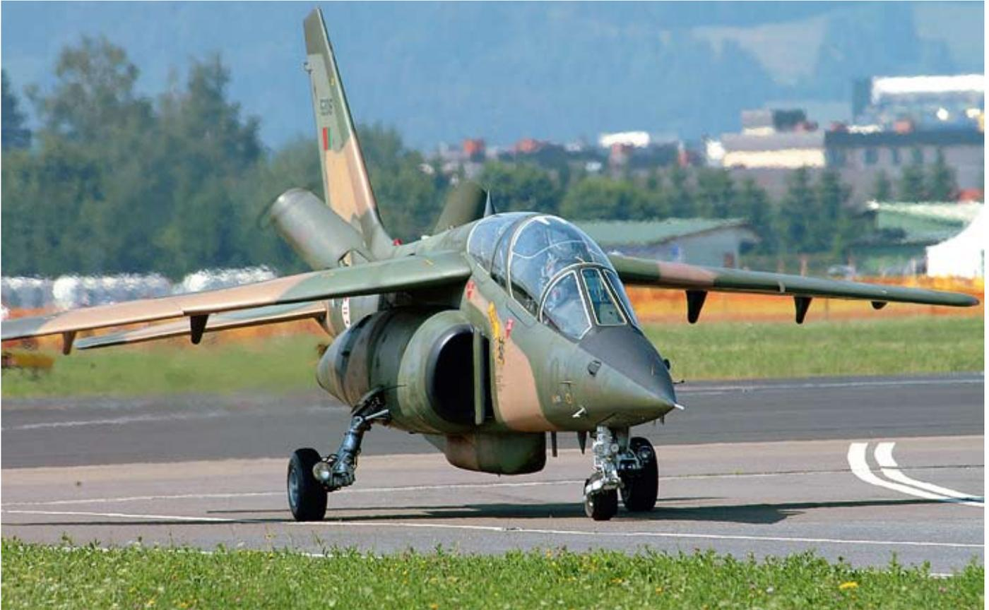
The Dornier/Dassault "Alpha Jet" – the first European mass-produced aeroplane with carbon fibre-reinforced plastic components
