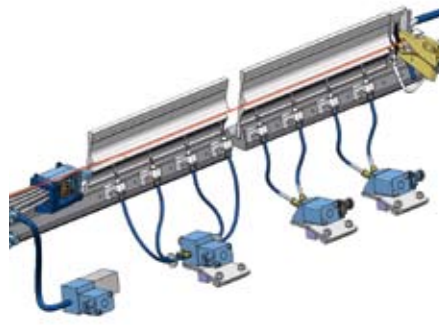
Reduced air consumption by way of 2 nozzles per valve
