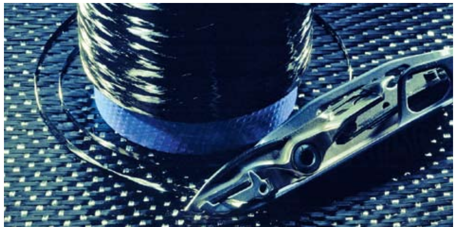
Woven carbon fabric – produced on a DORNIER rapier weaving machine
