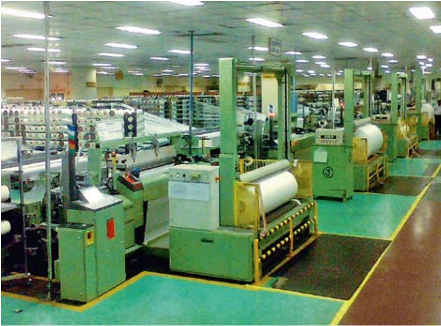
DORNIER tire cord weaving plant of SRF
