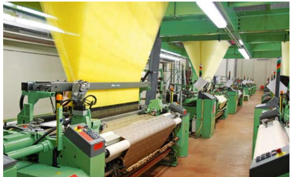
The modern weaving plant with DORNIER dobby and Jacquard weaving machines
