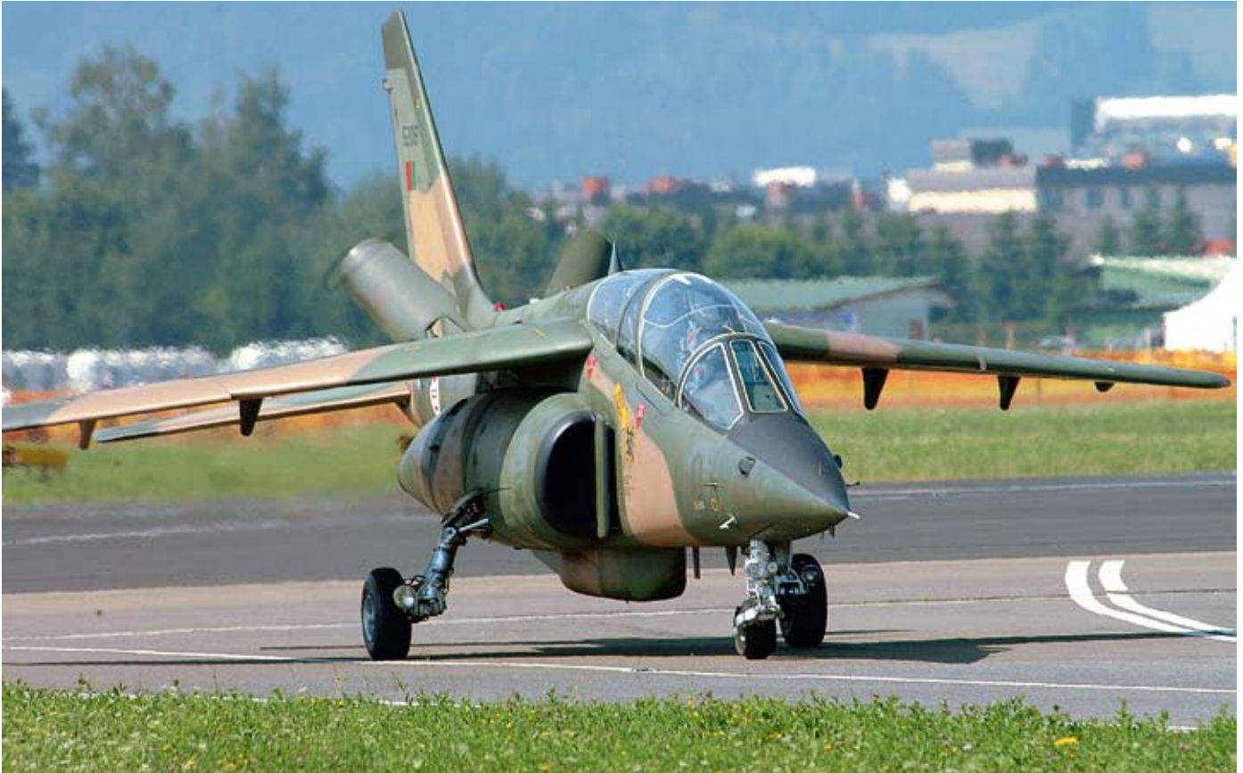
The Dornier/Dassault "Alpha Jet" – the first European mass-produced aeroplane with carbon fibre-reinforced plastic components
