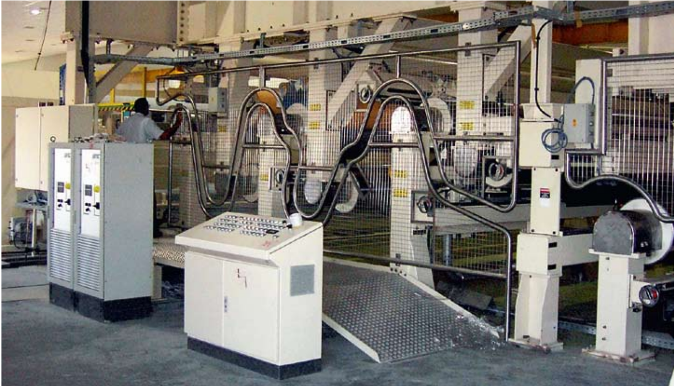
Take-up unit of a DORNIER film stretching machine at the SRF factory in Indore
