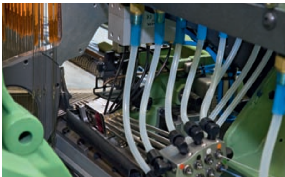
The new DORNIER PWC positive controlled filling thread clamp (patent applied)
