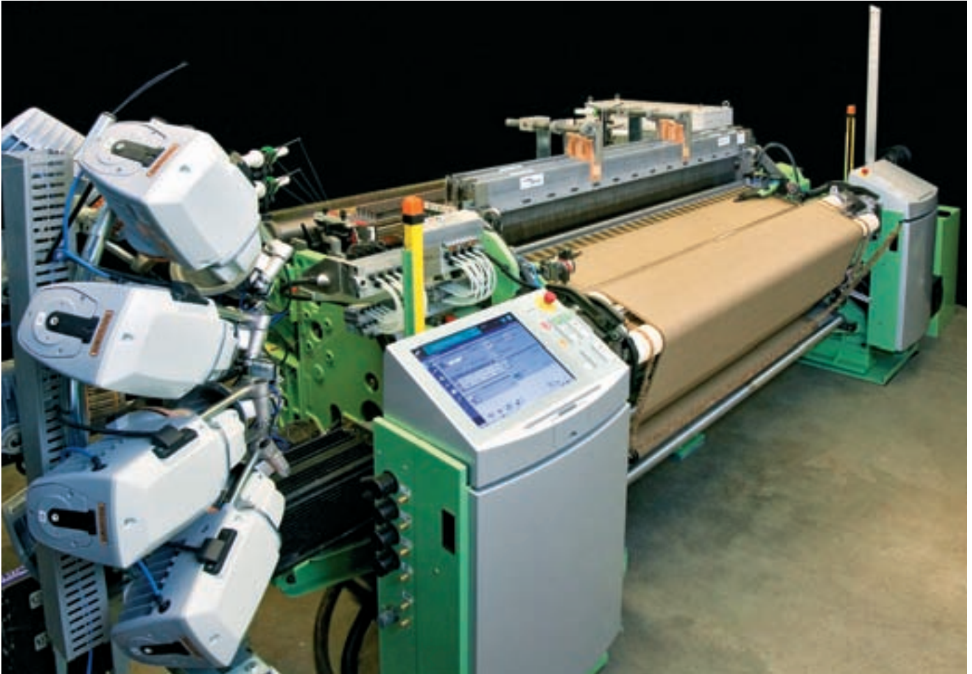
CLS "Concept Loom Study" – with new main drive concept "SyncroDrive" as well as the new electronic control and communication technology
