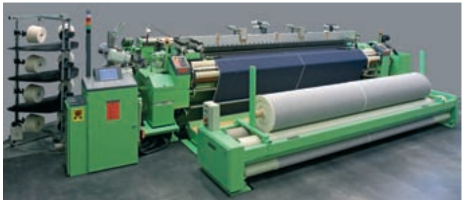
Stretch denim produced on DORNIER air-jet weaving machine with the usual width of 400 cm common today
