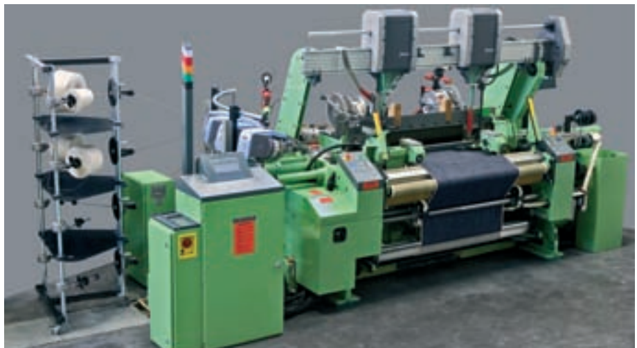
“Blue Mauritius Label” high-grade denim woven on a DORNIER rapier weaving machine
