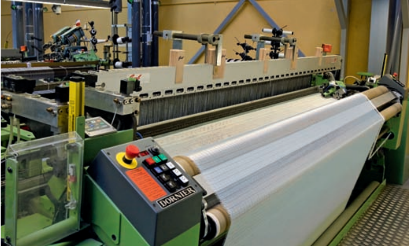
Polyester grid filter fabric on a DORNIER air-jet weaving machine at Nicolaus Weber GmbH
