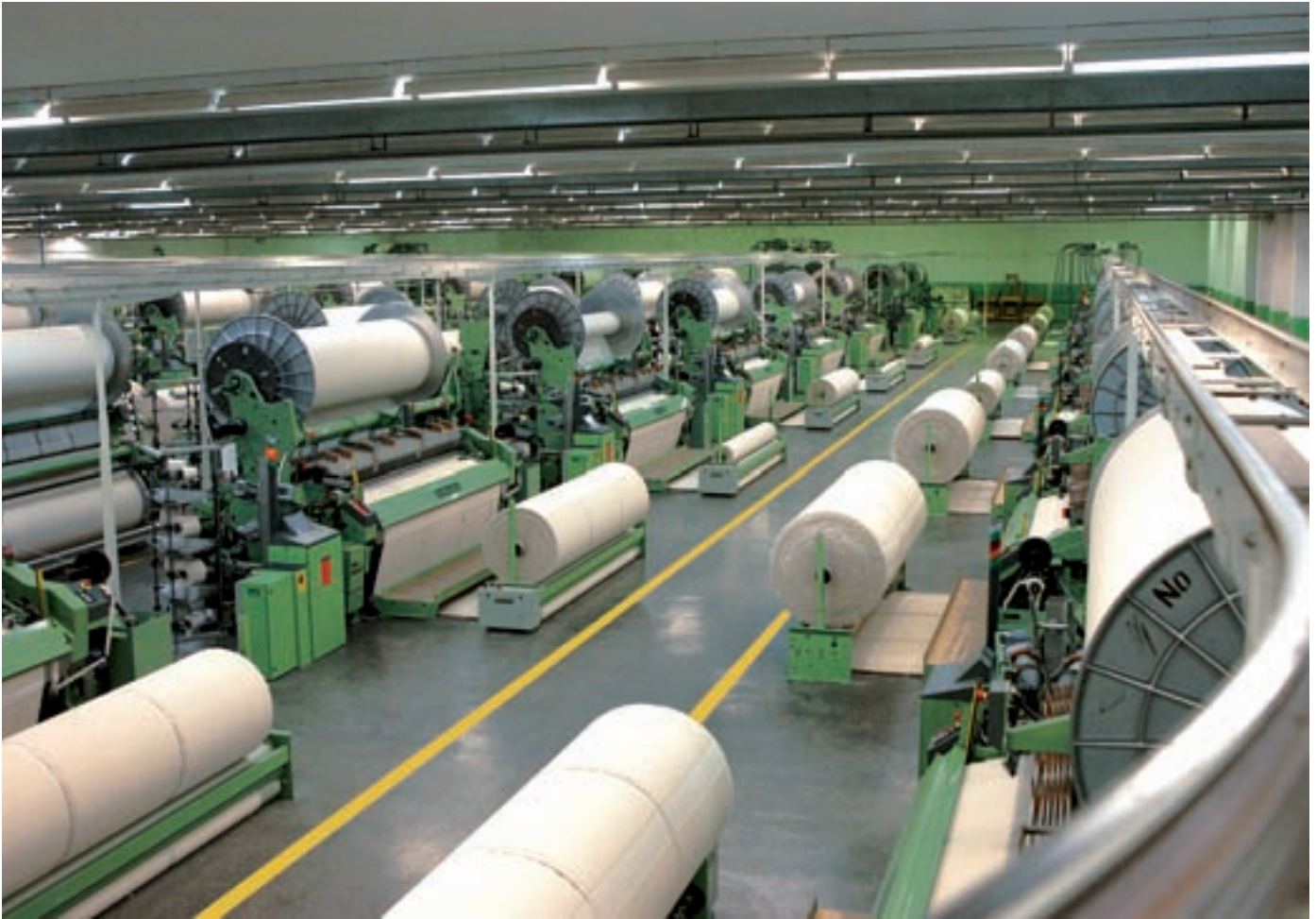
View in the weaving room of Indus Home Ltd. with the 48 DORNIER air-jet terry weaving machines already in production
