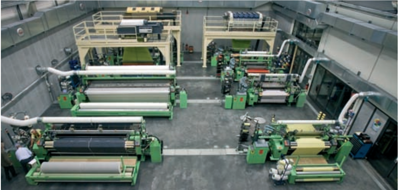
DORNIER LAB: Equipped with air-jet and rapier weaving machines of very different configurations
