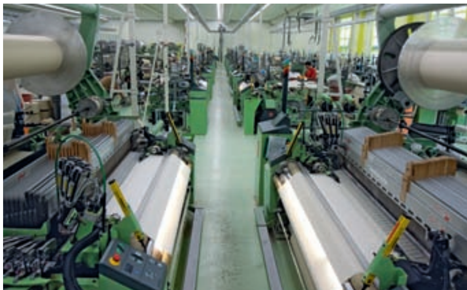
The DORNIER system family in use at Jenny Fabrics: In the foreground, high-shaft rapier weaving machines, in the background, high performance air-jet weaving machines
